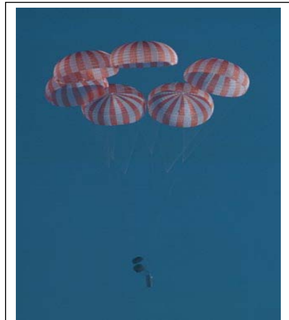
Figure 2-11: Six-Parachute Cluster Drop Test of First Stage Return
